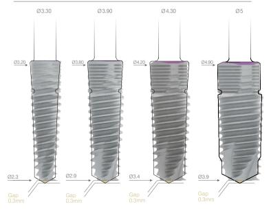
Implant and drill measurements
